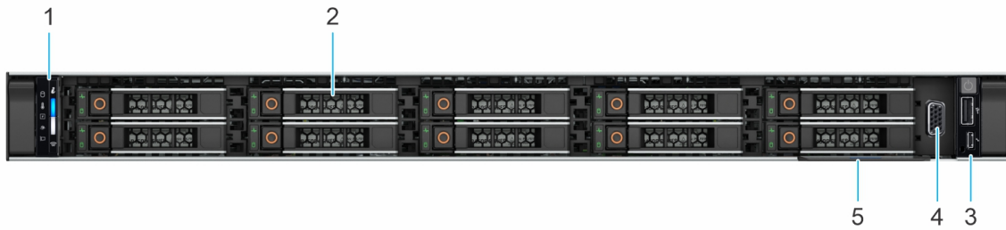
Figure 3. Front view of 10 x 2.5-inch drive system
